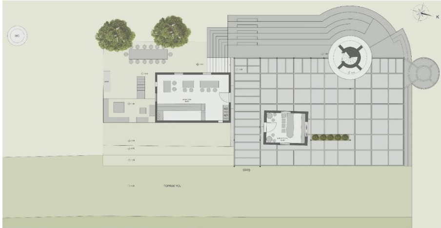
Fig. 7. Site Plan of the social area of the Eco-Village. The terrace and light-weight shelter above it integrates the operating light tower, dining area (former keeper's residence) and sales area(former depot) as well as the open-air social areas.
